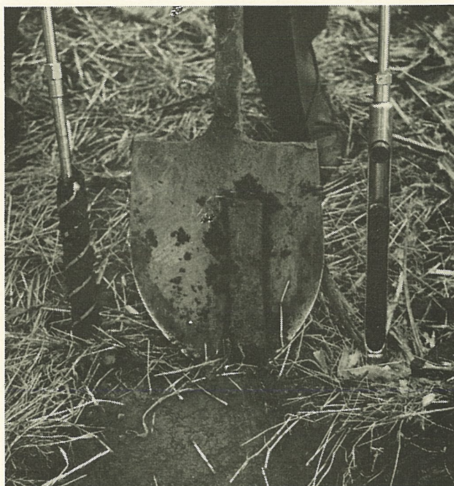
Figure 1. A soil probe, auger, or spade and knife should be used in sampling soils. The spade sample must be trimmed as shown.
